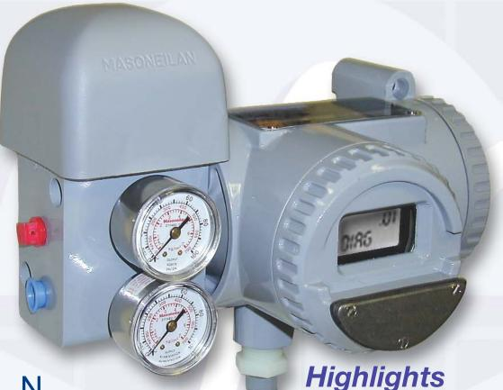
New and existing pneumatically actuated valves can be modernized with advanced control technology using Masoneilan's Smart Valve Interface (SVI). In addition to being a smart positioner, the SVI can also perform PID loop control. HART™ communication capability enables use of SVI with existing 4-20 mA wires.
