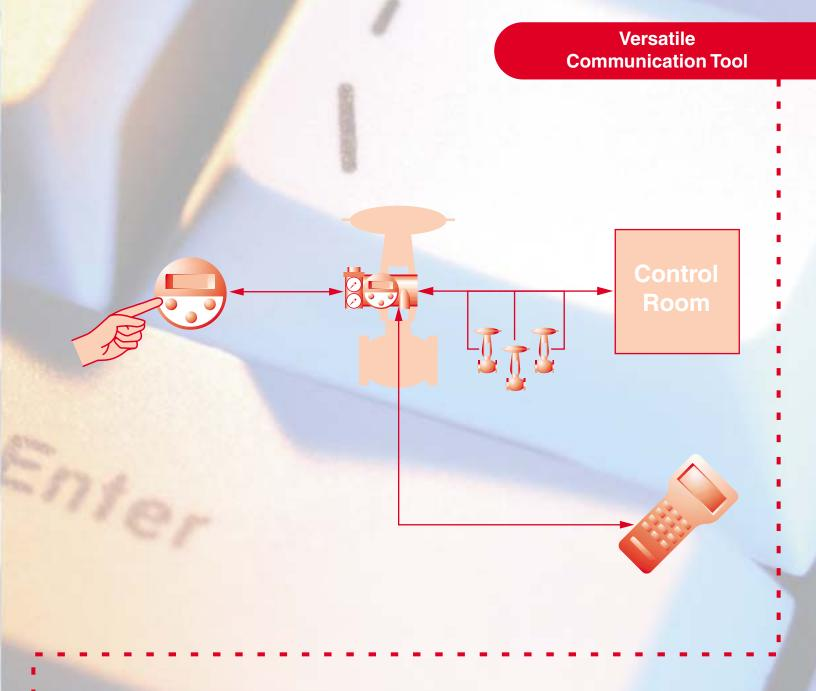
The SVI always provides the option for local or remote communication, even in hazardous environments.
