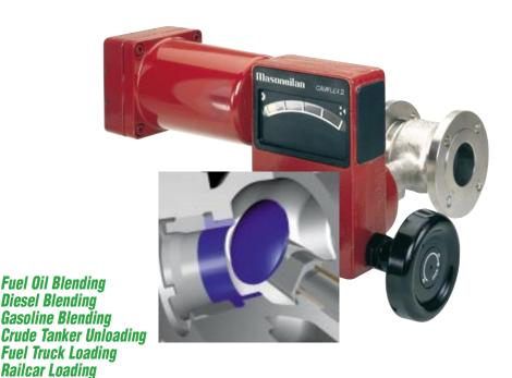
The Masoneilan® 35002 Series Camflex® eccentric plug control valve offers simplicity of design with enormous flexibility and capability. An optional soft seat design meets ANSI Class VI shutoff requirements. The Camflex design also includes the EF Seal as a standard packing configuration, which effectively minimizes hazardous emissions.
