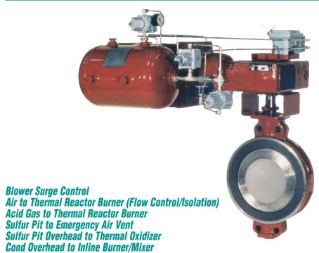
The Masoneilan\* 39002 Series High Performance Butterfly Valve (HPBV) is a heavy-duty automatic throttling control valve that incorporates tight shutoff (ANSI Class VI), lugged designs, heavy shafts, and optional spring diaphragm or piston actuation. The 39002 Series also includes an eccentric disc and shaft alignment, which improves the metal and energized PTFE seal ring performance. The 39002 Series is also provided with a steam jacket option to handle difficult liquid sulfur applications.
