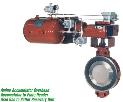
The Masoneilan 39002 Series High Performance Butterfly Valve (HPBV) is a heavy-duty automatic throttling control valve that incorporates tight shutoff (ANSI Class VI), lugged designs, heavy shafts, and optional spring diaphragm or piston actuation. The 39002 Series also includes an eccentric disc and shaft alignment, which improves the metal and energized PTFE seal ring performance.
