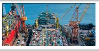
Offshore oil production facilities including over 50 wells, flow lines, risers, and two floating production, storage, and offloading vessels (FPSOs). Each FPSO produces 150,000 barrels per day and has a 2 million barrel storage capacity.
