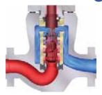
LincolnLog the unmatched anti-cavitation solution for high pressure liquid letdown.
